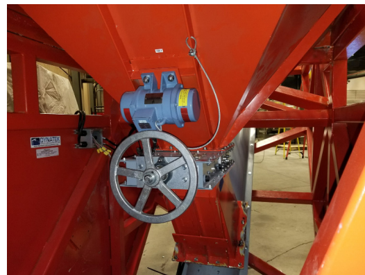
Rotary Electric Vibrator in use above a manual flow gate to rid the hopper of ratholed or hung up material.
